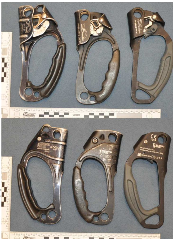
Obr. 2: Ruční blokanty Singin Rock Lift (rv: 2005), Singin Rock Lift (rv: 2005), Singin Rock Lift (rv: 2018)
