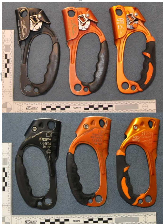
Obr. 4: Ruční blokanty Singing Rock Lift (rv: 2005), Timus Safety Ruční blokant (rv: 2007), Climbing Technology Quick Up+ (rv: 2019)
