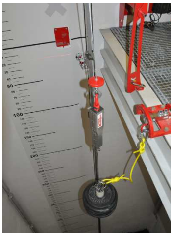
Fig. 6: Falling test mass during the figure eight loop test
